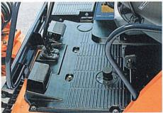
Easy-to-clean integrated molded resin floor
