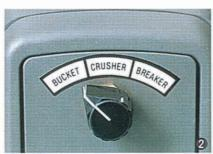
Extra Port that Sets Optimum Flow to Optional Attachment: The extra port is a hydraulic source for setting and delivering the optimum oil flow to optional attachment that is well matched with the front attachment. Attachment Mode Optionally Available: The attachment mode can be selected with the attachment selection switch according to the attachment used. This makes combined operation smooth.
