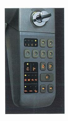
Power Selector: The power selector makes full use of the engine horse-power by sensing the changes in engine speed that occur with each new load. Depending on the job, you can select the mode which best suits your needs: P (Power) mode, E (Economy) mode, L (Low speed) mode, and I (low idle) mode.
