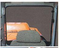
Curved Rear Window Glass: The cab rear window is curved and large enough to give excellent rear visibility. Low-profile engine hood helps increase rear visibility.
