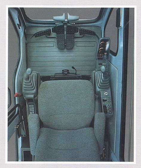
The Cockpit: Operator comfort and convenience are a top priority in the Super EX. Sit in the comfortable suspension seat, and notice how relaxed you feel. The seat can slide by itself, or together with the control levers and panel, to adjust to the proportions of any operator. This simultaneous seat/ lever movement also makes deep excavation easier and more efficient.
