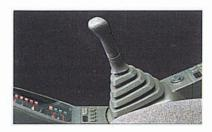
Ergonomically Designed Lever Grip: Lever grip, ergonomically designed, enhances pleasant human-touch control, minimizing operator fatigue.
