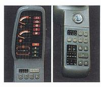
Easy-to-Read Monitor and Finger-Touch Switches: The monitor is curved for easy reading. Touch switches are resin-molded for dust protection. The engine speed control unit, which also functions as the power selector, can be controlled with one touch for simple operation, boosting operating efficiency.
