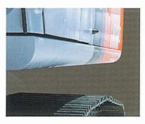
Rugged D-section Frame Skirt: Rugged D-section frame skirt, proven on the EX series, provides high resistance to deformation.
