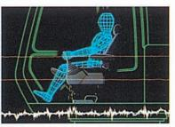
Low Noise and Vibration Design: The cab is rubber-mounted to absorb shocks and sealed to shut out noise. What's more, the cab is molded for improved rigidity to resist resonance.
