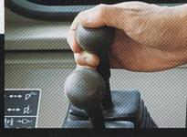
• Micro-Computer Controlled Transmission: Here advanced Hitachi technology enhances operating ease with features like the 2-Way Shift Switch: This button on the top of the grip for the lift arm control lever allows for quick shifting between 3rd and 2nd, and 2nd and 1st gears. Push the button and the transmission goes down a gear into 2nd or 1st gear respectively, push it again, or shift to in reverse, restores the selected gear. No other shift
