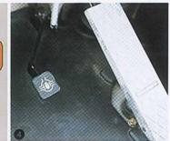
**1** Automatic Shifting: Just put the shift lever in the 4th gear and accelerate. Transmission starts out in 2nd gear, then shifts to 3rd and 4th gear as speed increases. This works well in transport or load and carry applications.
