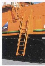
■ The retractable ladder. provided on one side of the basic machine for protection against damage, gives easy access to the cab.
