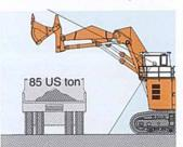
■ A high 6.1 m (20'0") operator eye level plus the forward sloping cab give good downward visibility. The vessel of the dump truck being loaded is clearly visible to the operator.
