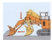
The renowned auto-leveling crowd mechanism, a Hitachi original, brings operating ease and increases job efficiency, by one-lever (left) control. This allows quick leveling and easy foundation digging, while reducing track wear.
