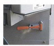
■ The emergency evacuation hammer is provided in the cab for getting out of the cab in the case of an emergency.
