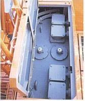
■ Centralized hydraulic oil filters make servicing easy. Oil spills during servicing are reduced significantly because filter elements can be removed upward. High-pressure line filters are also provided.
