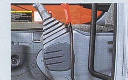
• Pilot-control shutoff lever, (locked)
