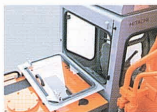
● Emergency evacuation window
