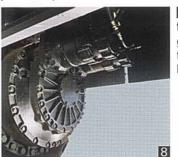
8 High-mounted compact travel motors stay clear of the ground. This design protects the travel motors from damage by rocks and rough terrain.
