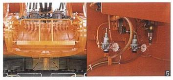
5 Auto lubrication system (option) is provided for front joint pins and swing circle. This eliminates cumbersome daily lubrication.
