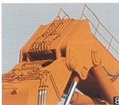
B High-pressure hoses at the link between boom and arm are well arranged and clamped to protect them from fraying
