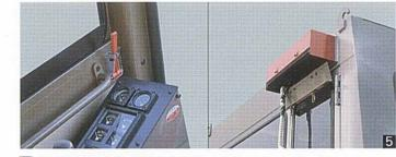
**Emergency evacuation hammer and emergency rope** are provided for getting out of the cab in case of an emergency.
