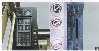
Easy-to-read monitors are ergonomically designed to allow for quick checking of machine conditions.
