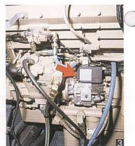
The electric engine governor (CENTRY™), teamed with a microcomputer, reduces fuel consumption and exhaust gas
