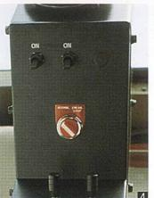
4 Emergency engine stop switch is provided inside the cab.
