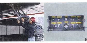
☑ The centralized lubrication system: Fast filling system (option) allows easy replenishing and change of fuel, engine oil, hydraulic oil, etc. from the ground. There is no need to bring a pail can up to the machine.
