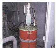
6 A grease drum can be replaced effortlessly. The compartment floor slides down to lower a drum for simple, easy replacement.
