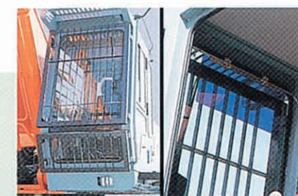
Cab front guard and sunvisor are optionally available for the pressurized cab with integrated headguard.
