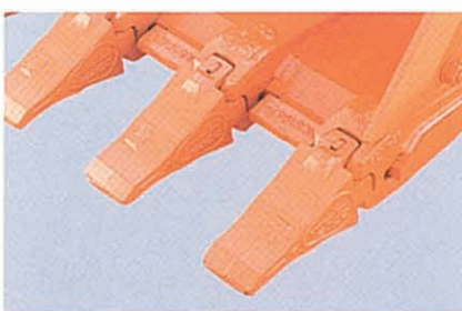
Big bucket teeth are utilized for rock excavation to prevent disengagement and increase wear resistance.
