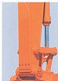
Damage prevention plate and square bars are provided at the bottom of the arm for protection against damage due to rocks caught during excavation.
