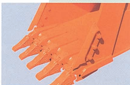
Strengthened Side Shrouds Side shrouds are enlarged and strengthened to reduce wear of bucket side plates.
