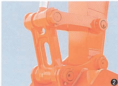
② Bucket link A is cast monolithically to resist torsion for added durability.
