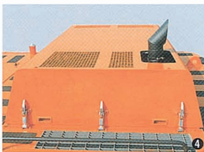
④ Three engine cover locks hold the engine cover securely, reducing its jolt.
