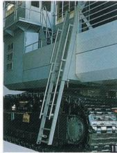
The retractable-type ladder is provided on the left side of the basic machine to reduce the possibility of accidental damage.
