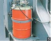
4 Centralized filtering of hydraulic oil filters makes servicing easy. In addition, oil spills are minimized during service due to vertical filter mounting.
