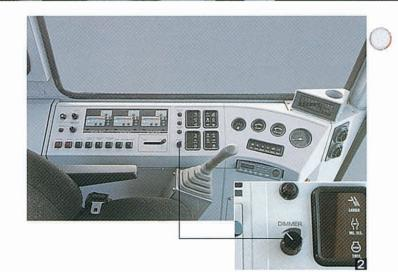
The monitor/switch panel is ergonomically designed to allow for quick reading of gauges and warning indicators.
