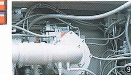
**⑨ Pump bulkhead** provided between pump and engine.
