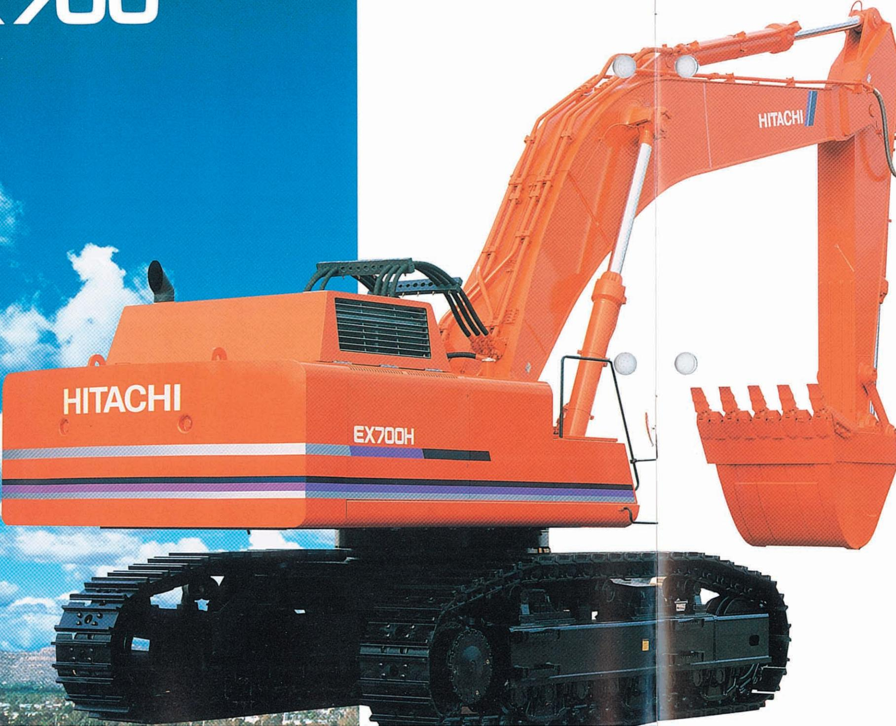
① **Improved E-P control** for optimum control of the engine and pump according to worksite conditions for higher productivity. Optimum power and speed are always right at hand for increased productivity and for reduced fuel consumption.
