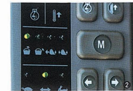
● Work mode selector gives a choice of four work modes—general purpose, trenching, grading and precision modes, at one touch of a switch. The precision mode also serves for powerful crane operation through the heavy lifting system.
