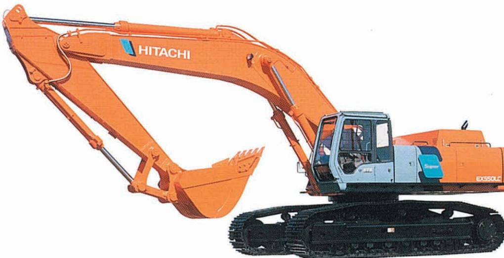
**① The reinforced front attachment** allows the EX550 to tackle tougher jobs than ever. The boom and arm are reinforced throughout, using thickened plates, oversized pins, strategically located bulkheads and backings, and marginal weld beads to resist stress concentration and counteract torsion. The result is ruggedness and durability for heavy-duty excavation and breaker operation. The bucket is built with improved wear resistance.
