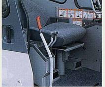
Pilot-Control Shutoff Lever to **Prevent Misoperation** When the Operator Gets in and out of the Cab
