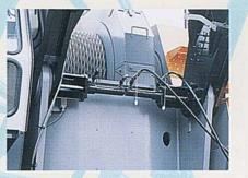
**Boom Foot Pin Connecting** /Disconnecting Device
