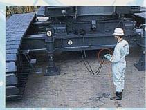
Self-Loading Device (Option) Using hydraulic jackup device, the basic machine can be quickly self-loaded onto a trailer.
