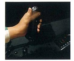
The electronic fuel control accelerator–fingertouch grip atop the swing lever–has been added to the conventional fuel control lever and accelerator pedal.
