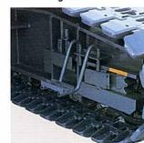
Sideframe step allowing easy access to machine
