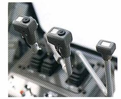
The newly-developed drum rotation sensor allows the operator to feel the starting of the drum with his hand.
