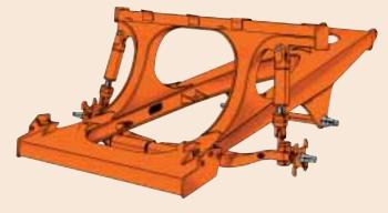
NEOCON struts outperform competitive strut designs by improving isolation, stability, and control. Improved isolation means reduced impact loading on the structural members of the machine and greater operator comfort, resulting in longer equipment life and increased productivity. Improved stability means more consistent dynamic response of the machine to fluctuating load energy, resulting in predictable machine performance. And improved control means better machine maneuverability.
