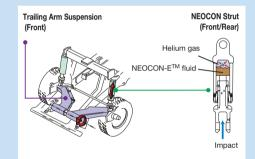
The ACCU-TRAC suspension design allows the front struts to be removed and installed without removing the trailing arms, brakes or tires. This relates to fewer tools and less labour required to perform the repair, which aims to reduce the amount of hauler
