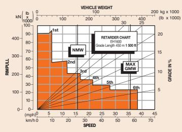
Diagonal lines represent total resistance (Grade % plus rolling resistance %). Charts based on 0% rolling resistance, standard power of engine, standard tires and gearing unless otherwise stated.
