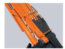
**Splitting Front Hose for Easy** Maintenance Front hose can be separated on
