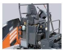
**Full-Open Type Side Cover** Full-open type side cover is provided for easier maintenance
