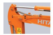
**Bucket Hose Stored in Arm** Bucket hose is stored in the arm to prevent damage.
