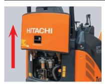
**Vertical Sliding Engine Cover** Vertical sliding engine cover enables easy maintenance even in confined spaces. When opened, the cover does not interfere with inspection or operation and provides easy access. (Patent pending)
