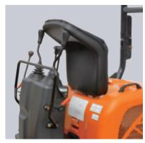
Folding/Retractable Seat Since the seat can be folded up, it can be used immediately after rainy weather, without the need for cleaning.
